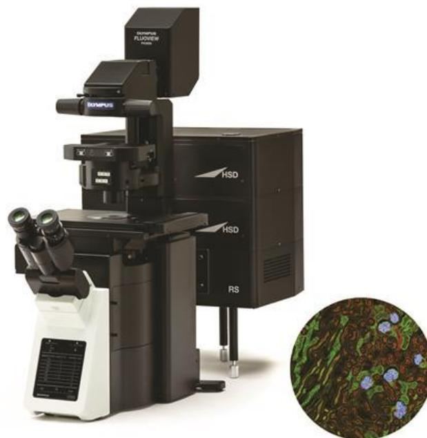
When used correctly, a confocal fluorescence microscope is an excellent tool for making quantitative measurements in cells and tissues. Its ability to block out-of-focus light and thereby perform optical sectioning through a specimen enables you to quantify fluorescence with very high spatial precision.
